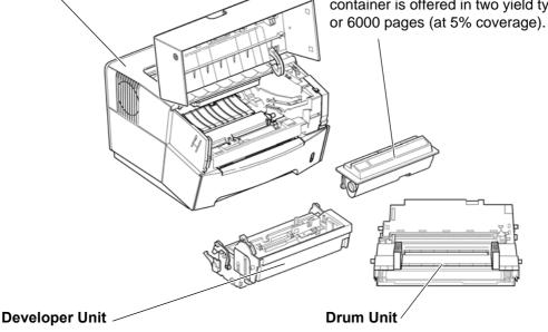
The developer unit should be removed to allow for cleaning tasks every time the toner container is replaced.
